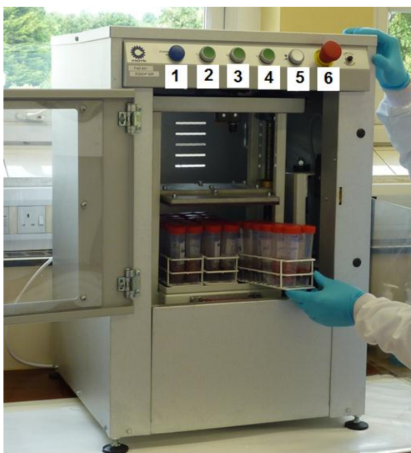
Fig. A. Vibrational extraction system used for unattended extraction. (1) operating light, (2, 3 and 4) shaking speeds, (5) start/stop and (6) emergency stop.
